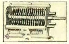
ting condensers. Known as the MTC series, they are available in both single and split stator units in capacities ranging from 20 to 530 mmfd., and in breakdown voltage ratings irom 1000 to 6000 volts. Thorough Isolantite insulation and a silver plated Beryllium contact wiper are used for low loss. The condensers are designed ior either panel or base mounting.
