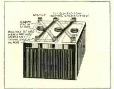
The binding posts strips, 3/4 inch wide. are of the self-tapping variety. H. D. HOOTON, Beech Hill, W. Va.
