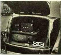
The transmitter is equipped for c.w., modulated c.w. and phone types of emission, which can be selected by a 3-position, 4-gang switch. By means of plug-in coils it has an unusually wide frequency coverage from 1500 to 60,000 kilocycles.
