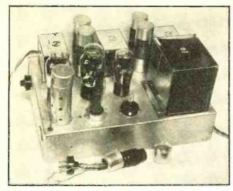
THE COMPLETED AMPLIFIER CHASSIS Illustrating the ship-shape layout for the new directcurrent, push-pull amplifier. Note the small "lamp-fuse" at the front of the chassis which gives ample protection.
