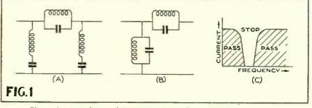
Figure 1. Two forms of hand-suppression filters and the transmission characteristic produced
