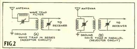
Figure 2. Band-suppression wave traps or filters connected to the antenna circuit of a radio receiver to eliminate interference from unwanted stations. (A) Series scave trap. (B) Shunt or parallel wave trap.
