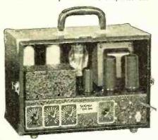
ploys the following type tubes: two 6F5's, one 6N7, and two 6L6's connected in pushpull in the output stage. It has input con-nection arrangements for 2 microphones and phonograph pick-up. The output impedance is 250 ohms.
