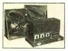
and operation. The output circuit has provisions for the connection of additional loud-speakers. The amplifier has a rated output of 35 watts peak and it employs 8 tubes in all, including two type 6L6's which are used in the power stage.
