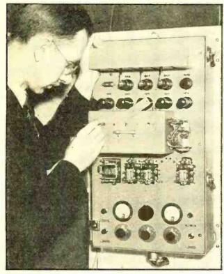
THE AUTOMATIC RADIO ALARM UNIT Engineer adjusting one of the sensitive electrical relays of the automatic "listener".
