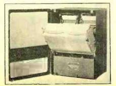
watt from the measured circuit. The double photo-electric recorder can be applied wherever simultaneous readings are desired. In some cases this immediately cuts testing time in half and in others it aids materially in discovering unusual relations between two variable electrical quantities.
